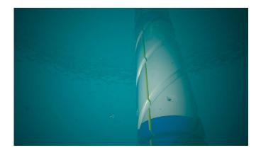
Joint handling times and running methodologies during riser deployment and retrieval are equivalent between Magni DRBM HG and traditional buoyancy designs, resulting in increased personnel safety, higher efficiency and a more robust solution compared to traditional VIV mitigation equipment.
