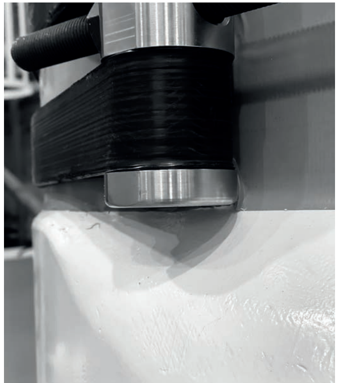
Strap and tensioning assembly under load
