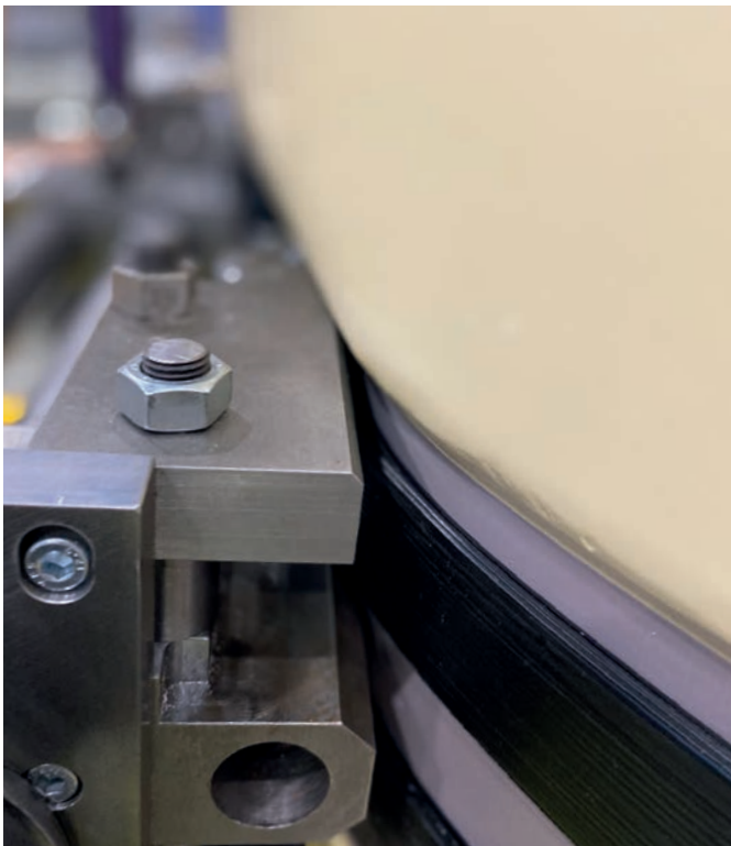
Strap being tensioned by the installation tool
